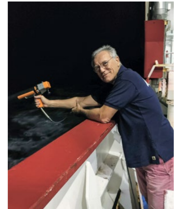
XBT launch from the deck of the S.A. Agulhas II © Jean-François Ternon - IRD / Monaco Explorations.
