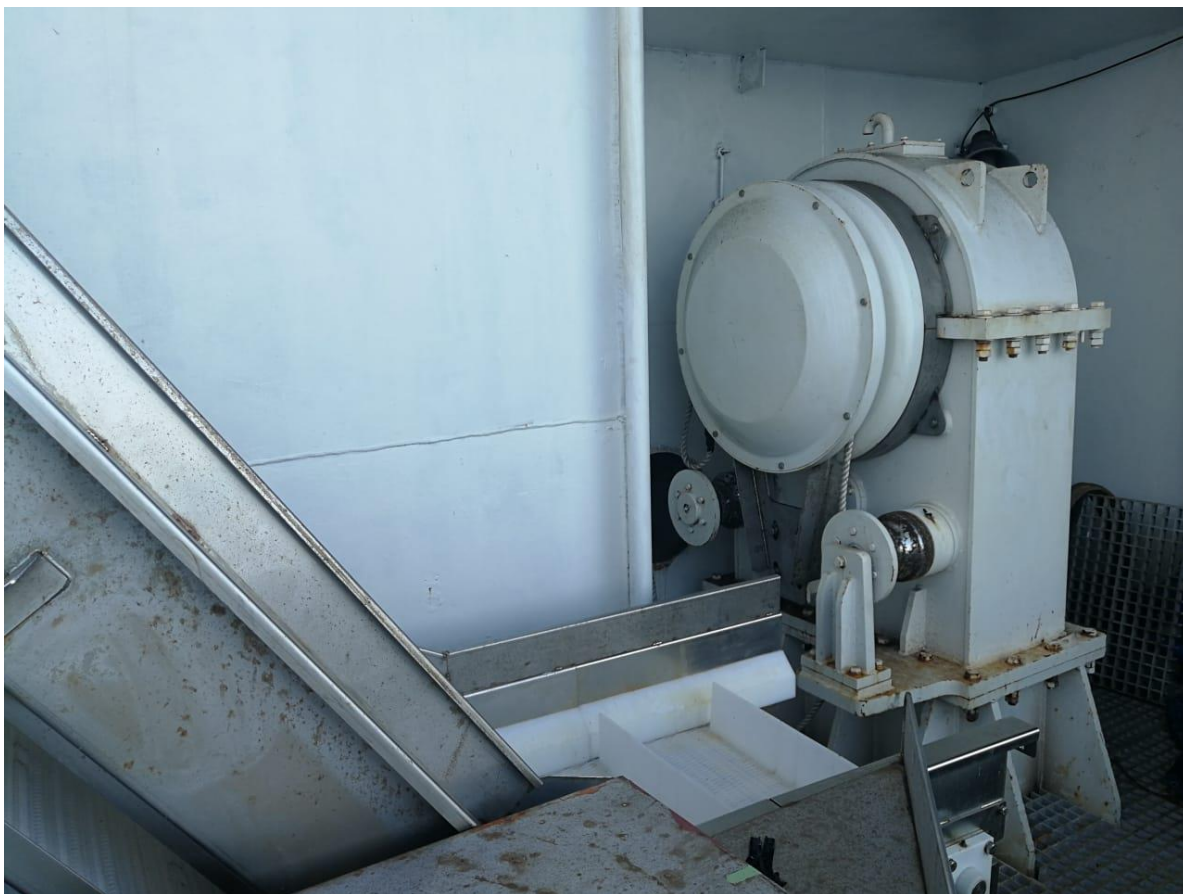
Figure 6: Hydraulic winch and transporter
