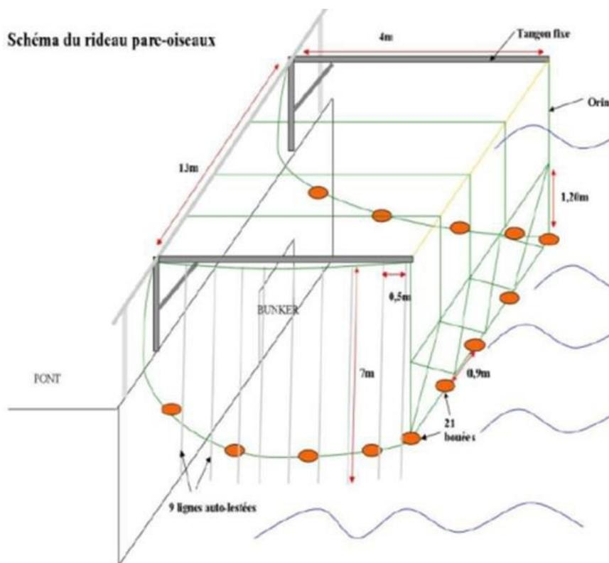
FIGURE 4: BRICKLE CURTAIN DEVICE
