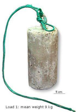
Granite / cement block in the polypropylene line, 8 mm Ø, y 25 m length
