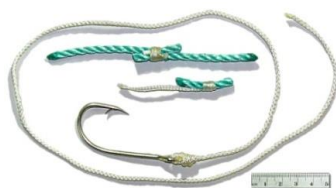
Hook line, nylon 3mm Ø.
