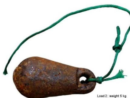
Standard iron weight in the polypropylene line, 8 mm Ø, y 25 m length
