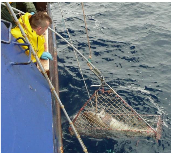
Figure 7. Lifting aids for supporting the fish onboard
