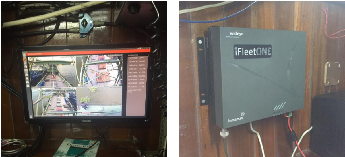
Figure 4 Processors and connectors for satellite data transmission
