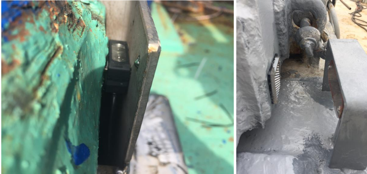
Figure 3 the electronic sensors attached to winches, cranes and door of fish hatch to detect fisheries activities.
