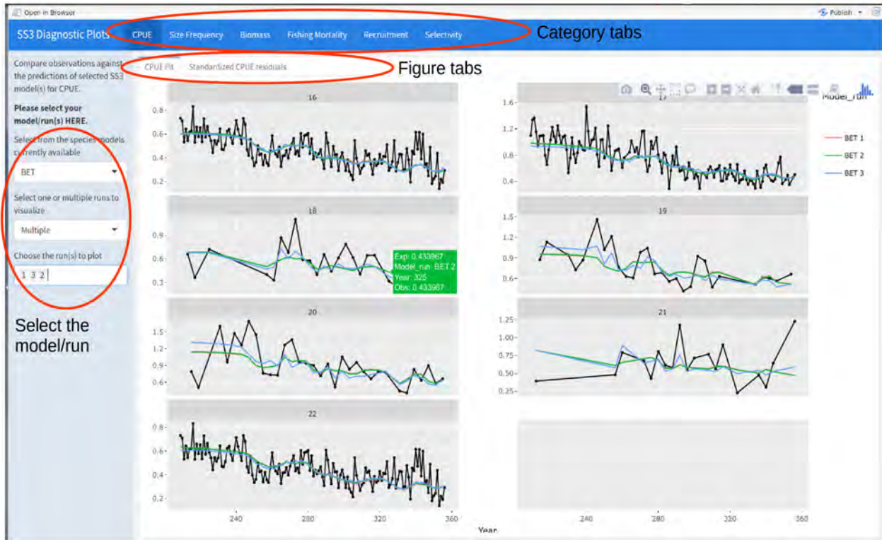
Figure 5: The R Shiny allows users to visualize the results of current or past model runs, allowing runs to be overlaid to compare results. The Shiny for the IOTC SS3 VRE includes diagnostic plots aimed at comparing between observations and predictions of the model(s). The plots currently included are CPUE observations versus predictions, standardized residuals of CPUE, size frequency plots of aggregated length frequency, and mean length and weight distributions, spawning stock biomass, fishing mortality, and recruitment variations. This visualization tool is possible due to the standard NetCDF data output, enabling the tool to read and plot different data files using the same code.
