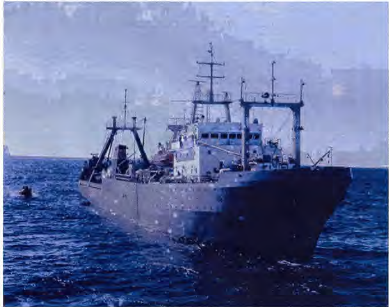
RTMS R.V. Zvezda Sevastopolya . These Super Atlantik types were built at Stralsund in East Germany by Volkswerft from 1971 to 1979; 95 vessels of this class were built. They had dimensions of 1988/2063 dwt; 3000/3977 gross tons, 1780/1830 net tons and a LOA of 102 m. They were powered by an 8-cylinder Dieselmotorenwerke 3880 bhp engine giving 15 knots (Greenway 1980).
