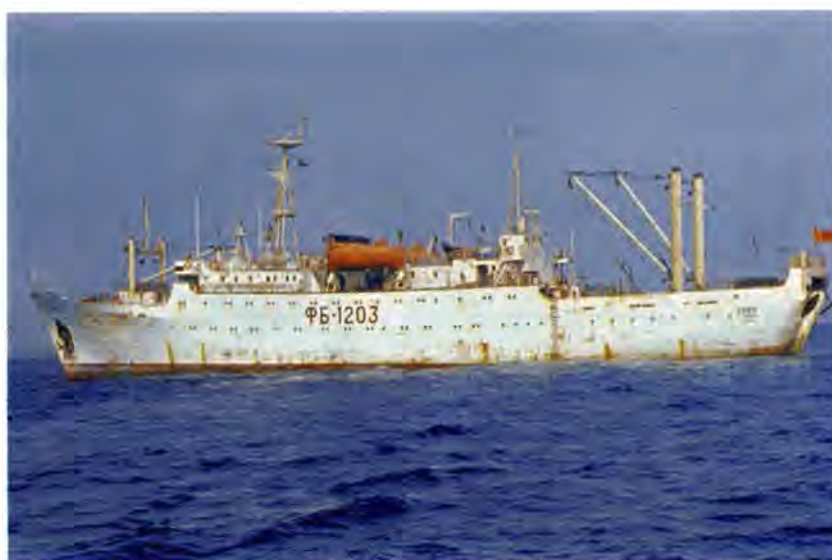
The BMRT fishery research vessel, F.R.V. Akademik Knipovich F.R.V. 'Skif' , used in Southern Indian Ocean surveys. This vessel's design was based on the Mayakoskiy type factory trawler. The Nicolaev and Baltiya shipyards built 109 мзяковский-class fishing vessels between 1958 and 1969. They have dimensions of 1519/1300 dwt, 3162/2691 GRT) (Greenway 1980).
