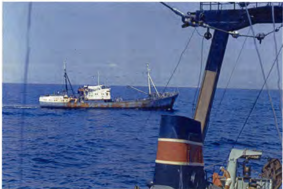
Fishing vessel of the "Mayak" SRTM class used in Southern Indian Ocean exploratory fishing. These "Mayak" class side-trawlers used a 25 m trawl, had a trawl drum capacity of 570 m, LOA 54.2 m, speed of 11.6 knots, 929 GRT, main engine 800 hp, crew of 30 and a 33 day at-sea endurance. Freezing capacity was 6 t/day at -18°C (Anon. 1968).
