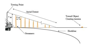
1. The aerial extent of the streamer line, which is the part of the line supporting the streamers, is the effective seabird deterrent component of a streamer line. Vessels are encouraged to optimise the aerial extent and ensure that it protects the hookline as far astern of the vessel as possible, even in crosswinds.
