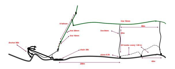
Figure 1b.- Fixing system of the Spanish BLL and first section of the rig.
