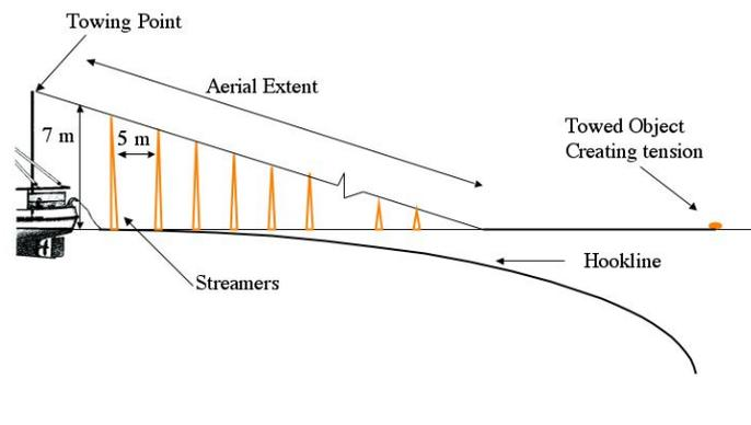
1. The aerial extent of the streamer line, which is the part of the line supporting the streamers, is the effective seabird deterrent component of a streamer line. Vessels are encouraged to optimise the aerial extent and ensure that it protects the hookline as far astern of the vessel as possible, even in crosswinds.
