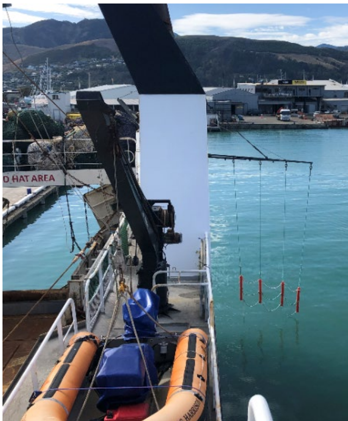
Figure A4-1: Bird baffle deployed. Seabirds are impeded from flying round the stern of the vessel.
