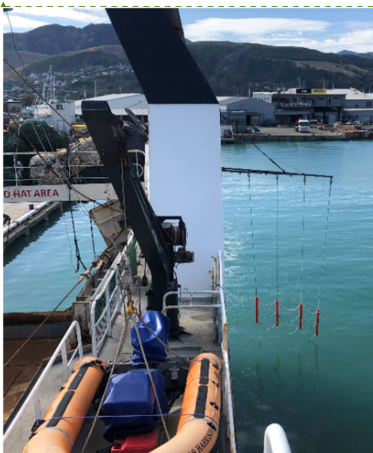
Figure A4-1: Bird baffler deployed. Seabirds are impeded from flying round the stern of the vessel.
